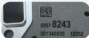
Marking on rough casting
