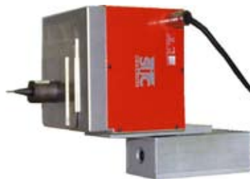
Z axis 50 mm / 2 inches to 250 mm / 9.84 inches stroke
